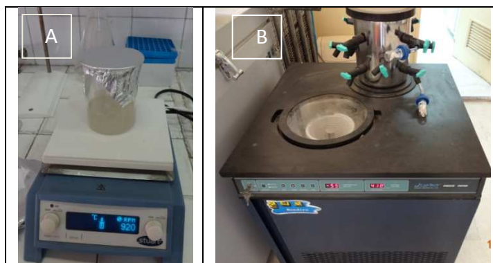
Figure 4. (A): dissolving chitosan powder in acetic acid solution with magnetic stirring. (B): lyophilizing the chitosan with freeze-dryer
